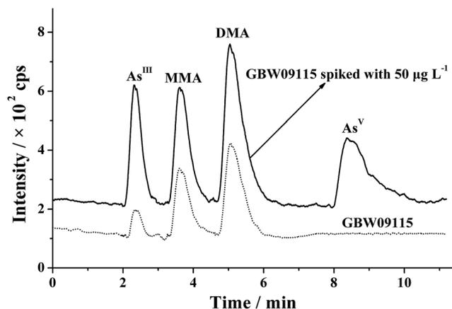
Fig. 5 Typical chromatograms of arsenic species in GBW09115 as well as the spiked solution (spiked with  $50 \mu\text{g L}^{-1}$ ). An isocratic elution was performed at a mobile phase flow rate of  $980 \text{ nL min}^{-1}$ .
