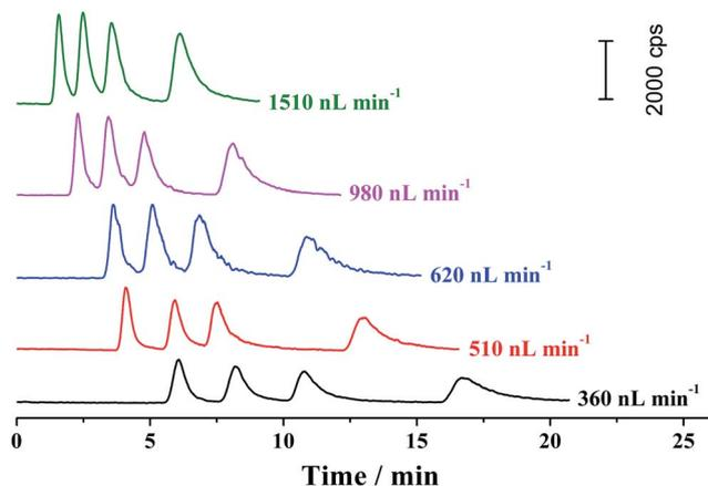
Fig. 4 Chromatographic separations of  $\text{As}^{\text{III}}$ ,  $\text{As}^{\text{V}}$ , MMA and DMA in  $500 \mu\text{g L}^{-1}$  by nanoHPLC-ICP-MS at various mobile phase flow rates. Peaks are in the increasing time order of  $\text{As}^{\text{III}}$ , MMA, DMA and  $\text{As}^{\text{V}}$ .
