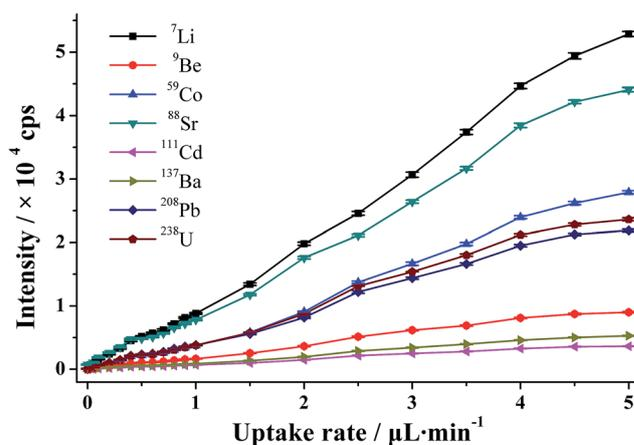
Fig. 3 Signal intensity as a function of sample uptake rate for the nanoflow nebulizer operating at a nebulizer gas flow rate of 0.88  $\text{L min}^{-1}$ , and the concentration of the multi-element solution was 10  $\mu\text{g L}^{-1}$  in 1%  $\text{HNO}_3$  for each element.
