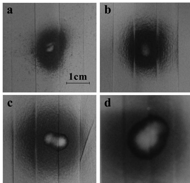
Fig. 2 Comparison of the aerosols generated by the d-NN ((a) 500  $\text{nL min}^{-1}$  and (b) 5  $\mu\text{L min}^{-1}$ ) and d-CMN ((c) 500  $\text{nL min}^{-1}$  and (d) 5  $\mu\text{L min}^{-1}$ ).
