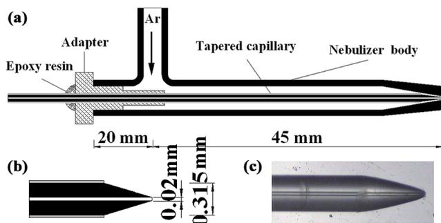
Fig. 1 Schematic diagram of the demountable nanoflow nebulizer (a), enlarged diagram of the nozzle (b) and the photograph of the fabricated tip (c). The dimensions are given in mm.
